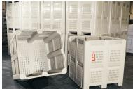
Reduced cooling costs Superior ventilation and tighter stacking means faster cooling in a CA room.
