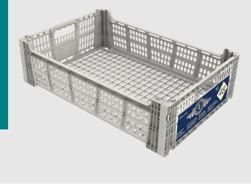
The single-piece, injection-molded MacroTote 5-FV with living hinges has been designed to be extremely lightweight, collapsible, and resuable, makign it one of teh best new totes on the market for one-way shipment of produce. Transferring weight down the corner columns when stacked, the full totes can be stacked 5 down, 10 high per pallet, and once collapsed, can be returned with 175 totes per pallet.
