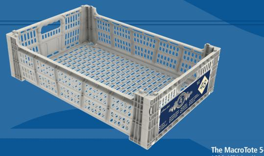
The single-piece, injection-molded MacroTote 5-FV with living hinges has been designed to be extremely lightweight, collapsible, and reusable, making it one of the best new totes on the market for the one-way shipment of produce. Transferring weight down the corner columns when stacked, the full totes can be stacked 5 down, 10 high per pallet, and, once collapsed, can be returned with 175 totes per pallet.
