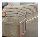
Empty plastic bins can be nested when shipped. The wood frames are shipped separately in flat kits to be assembled at the receiving site. Thus, the lowest delivery cost of any plastic bin on the market can be achieved.
