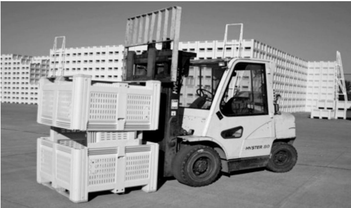
Photo #1: Removing or Placing Upper Bin in Nest
